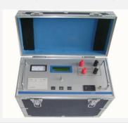
The winding resistance tester is an essential test project when the transformer transfers, repairs and changes tap-switch. Measuring DC resistance of transformer winding, you can check out weld or connection quality of down-lead, the winding inter-turn short circuit or open circuit, and whether tap-changer is well contacted.
