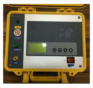
This Insulation resistance tester is used for aboratory or field testing insulation test, and it is dedicated to the measurement of water-cooled generator test. There is high-precision micro-current measurement system and digital boost system euipped inside. The test could be done by just using a high-voltage line and a signal line connecting the test product. Automatic measurement, the results from the large screen liquid crystal display, and store the results.
