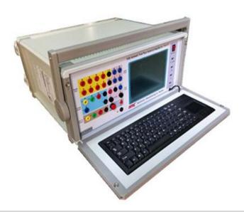
The instrument is the newest generation of relay protection testing system. It meets all the requirement of field tests. The tester employs DSP and Windows XP system, easy and fast to operate.
